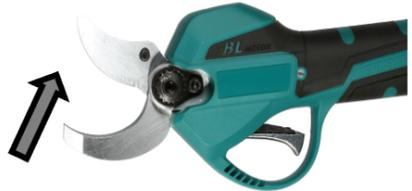
4. Remove the hex bolt near the shear blades with the hex wrench by turning it anticlockwise. Remove the blades tightening nut near the shear blades with a suitable wrench or alike by turning it anticlockwise and take out the washer.
