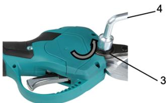
5. Remove two bolts near the shear blades with the hex wrench by turning anticlockwise.
