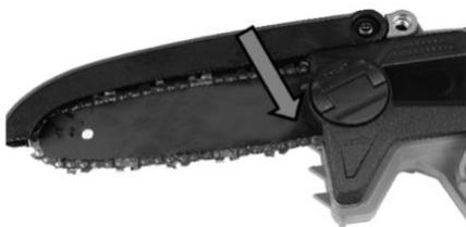
**⚠ CAUTION:** Make sure that the saw chain does not loosen at the lower side and the saw chain fits snugly against the lower side of the bar.
