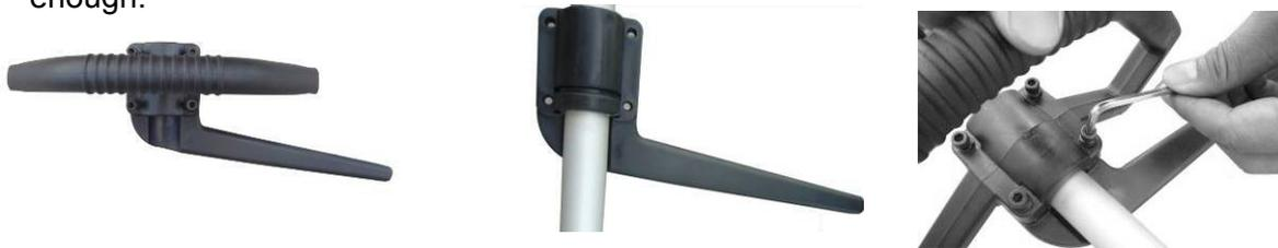
4. Assemble the safe guard. Release hex screws on safe guard fixed base, and then fix the safe guard with hex key and wrench enclosed as standard accessories for tightening the nuts enough.
