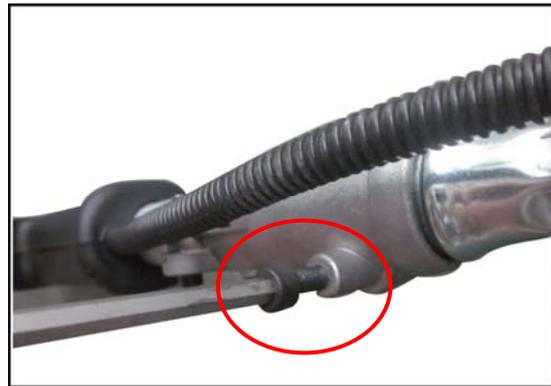
2. Connect throttle cable and switch on/ off wire.
