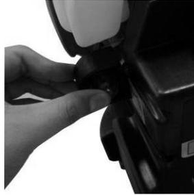
2. Turn the engine switch to the ON position.
